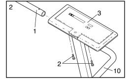
3. Insert a 5/16" x 2 3/4" Bolt (49), with a 5/16" Washer (26), through the lower end of the Right Handrail (10) and into the Frame (59). Reach under the Frame and tighten a Flange Nut (48) onto the Bolt.
